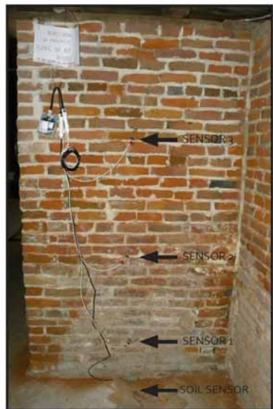
Figure 2: Photograph showing the testing assembly and installed temperature, relative humidity and a soil moisture sensors.
